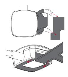
**9** Remove backing of adhesive on the FlexSensor in preparation for attaching to back of watch.
