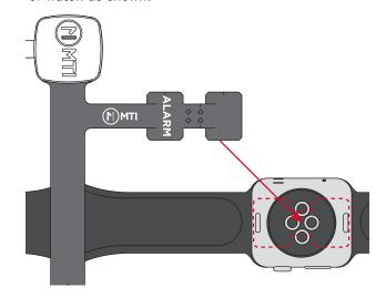
11 Turn watch over, wrap FlexSensor housing around watch band.
