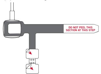
Firmly press FlexSensor adhesive side down on back of watch as shown.
