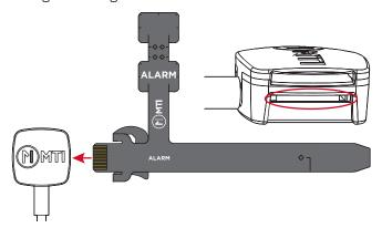
**8** Remove backing of adhesive and press firmly onto the underside of anchor housing.
