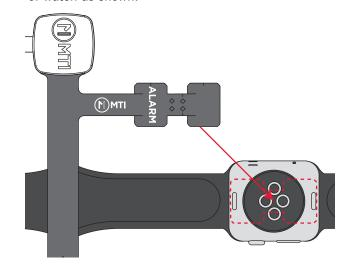
Turn watch over, wrap FlexSensor housing around watch band.
