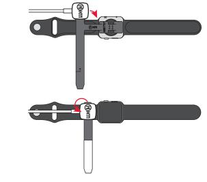
Wrap loop around and insert end of loop through anchor housing. Tighten FlexSensor, remove backing of adhesive and adhere to underside of sensor. There may be some excess material at the end which may be trimmed off. Remove Intellikey from Alarm Module to arm system.
