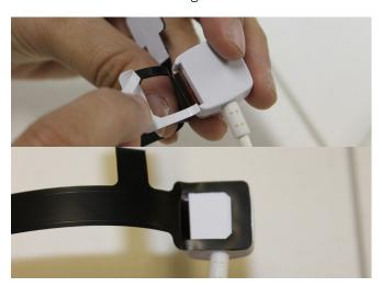
Remove backing of adhesive on the FlexSensor in preparation for attaching to back of watch. Firmly press FlexSensor adhesive side down on back of watch as shown.
