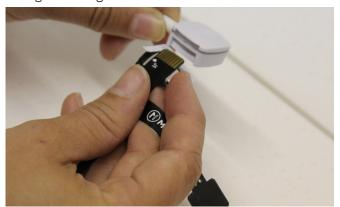
2 Remove backing of adhesive and press firmly onto the underside of anchor housing.
