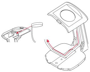
Slide the other half of the watch stand into place as shown. A slight clicking noise will indicate the two halves are in place. Secure with a screw and Double-Sided System Tool as shown. Plug in the Apple Inductive Charger.
