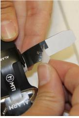
There may be some excess material at the end which may be trimmed off. Remove Intellikey from Alarm Module to arm system.
