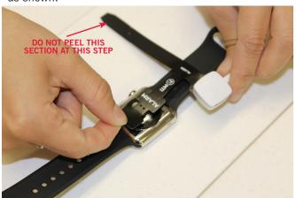
Turn watch over, wrap FlexSensor housing around watch band.
