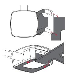
**9** Remove backing of adhesive on the FlexSensor in preparation for attaching to back of watch.
